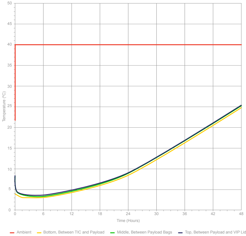
Golden Hour Medic, Unit 3, Thermal Performance (Control Set: 40°C Constant Ambient Profile, -18°C TIC Conditioning, 15 Minute TIC Staging at 22°C) (2 Ea. 500ml, H 2 O Bags, 5°C Payload Conditioning) Source: Pelican BioThermal, Lab 06 January 2017
